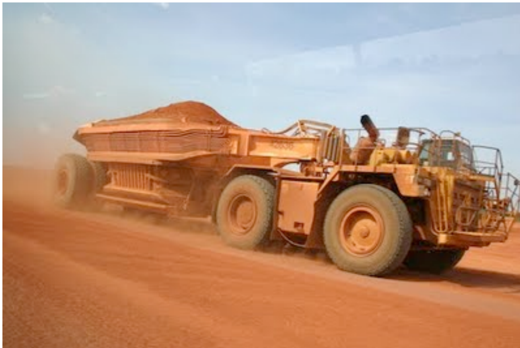
BELLY LOADER PASSING BY WITH 170 TONNES OF ORE
