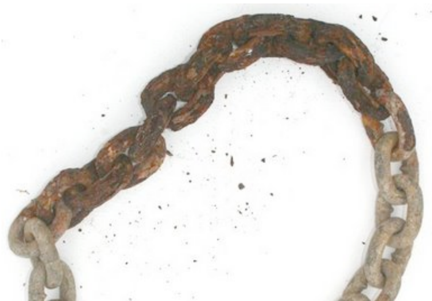
THE EFFECT OF SPRAY PAINT ON A GALVANISED CHAIN
