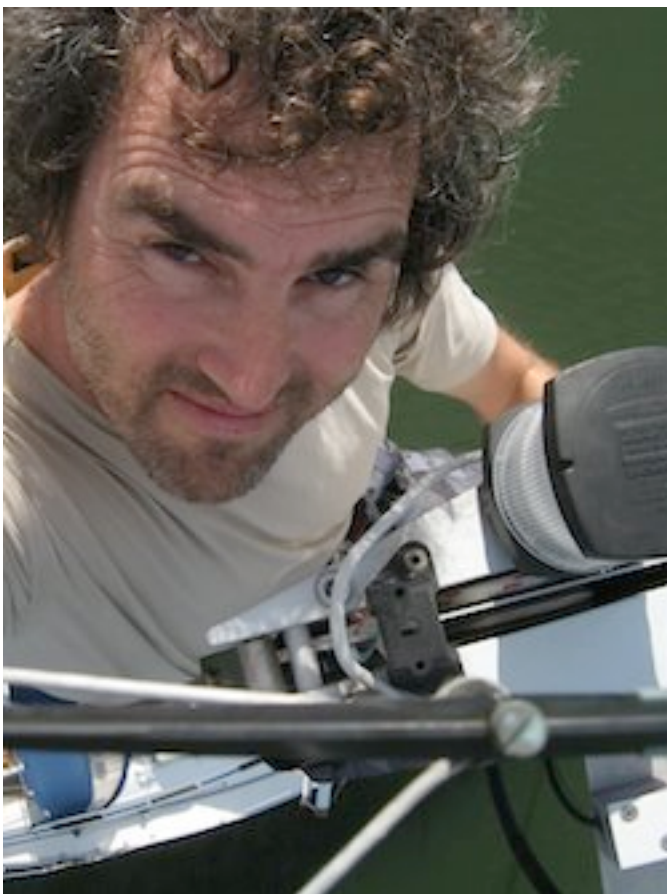
REPLACING THE MASTHEAD LIGHT
